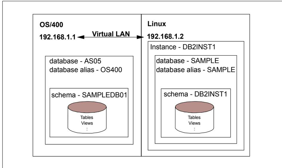
Figure 3-6 The system environment for the sample programs
